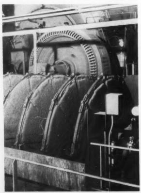
**REGRINDING AND FILTERING** are key steps to produce concentrate for pelletizing. Disc filter in front of regrind mill.
